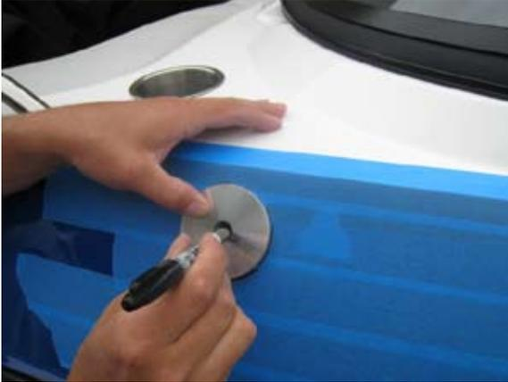
Once the desired position is achieved, place one of the large nylon whasers over the piece of tape and trace around it with a permanent marker.
