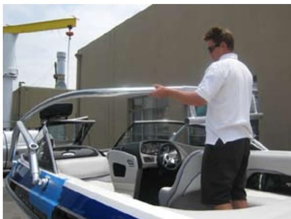
Do the same for the rear arms. It is important to try to keep the top section centered on the boat during this process.
